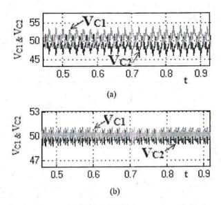
Figure. 9 Z-T NPC-MLI DC-link capacitors balancing simulation results; (a) Conventional ZSVPWM,(b) proposed ZSVPWM.I
