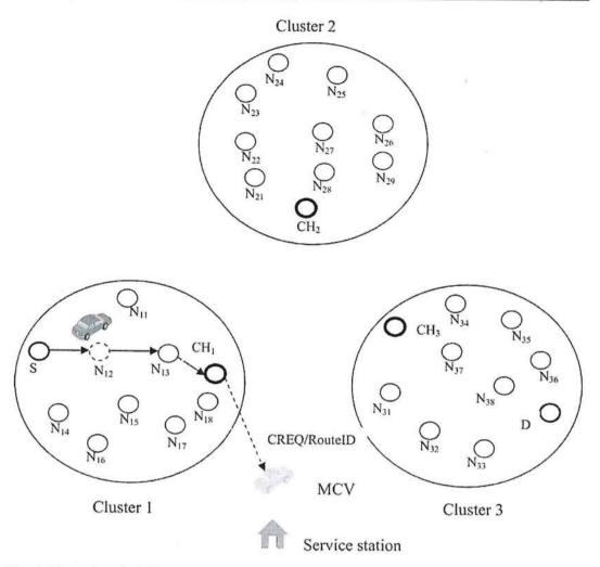
Fig. 4 Cluster-based wireless energy transfer (CWET)
