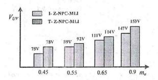
Figure.13 Experimental results; line voltage comparison between I-type and T type Z-source NPC-MLI
