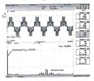
Figure. 10 Experimental line voltage (V<sub>LINE</sub>), and its respective THD spectra at m<sub>a</sub>=0.907.
