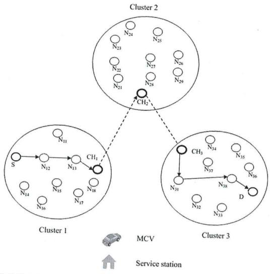
Fig. 2 Cluster-based routing
