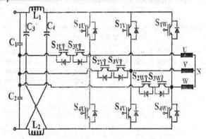
Figure 1 Topology circuit diagram of three-phase three-level Z-source T-NPC-MLI
