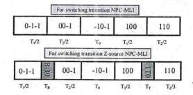
Figure.3 switching transition in linear modulation region for NPC-MLI and Z-source NPC-MLI
