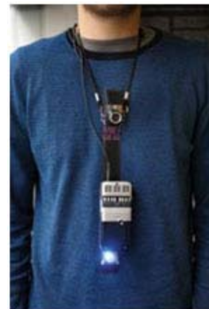
Prototype Equipped With Pocket Projector, Mobile Components, Mirror, Colour Markers, and Camera
