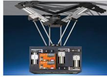
also modular in design, giving it flexibility in assembly and maintenance. Speeds are limited to 60 picks-per-minute
