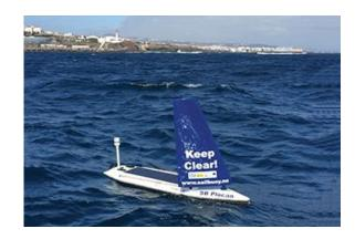
The Sailbuoy is loaded with echo sounders and atmospheric and water quality sensors for industry and scientific uses. Image: Sailbuoy
