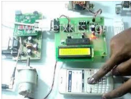
Then a micro-controller is used to detect these signals and facilitates the operation of motors which will then open/ close the gate. You can use IR sensors for detecting the train movement, micro-controller like 8051, 8052, Arduino Uno to act as the brain of the system and D.C motors to operate the railway gates.
