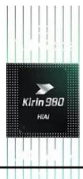
**Technology:** CMOS Die 74.13mm<sup>2</sup>**Cores:** 8**Word Size:** 64 bit**Threads:** 8
